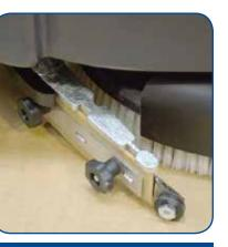
Parabolic squeegee, easy rubber blades replacement. The floating brush plate and squeegee grant the right cleaning pressure on any type of floor.
