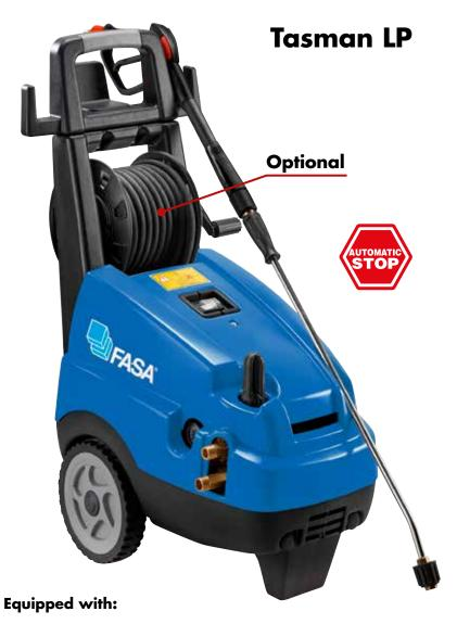
• 4 poles electrical motor (1450 RPM) with thermal protection and water cooling • Three ceramic coated pistons,(full ceramic pistonsonly for Tasman 1713) brass linear pump head with built-in by-pass valve. • Suction and delivery S. S. valves. • Low voltage and delayed Total Stop (three phase models) • Detergent tank (2,8 lt.). • Pressure regulator. • Glicerine pressure gauge. • Hose-reel (on request)
