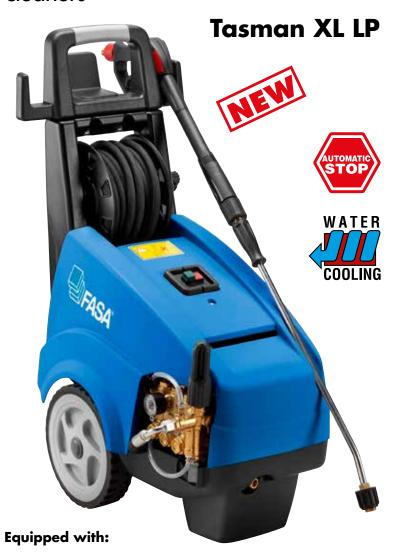
• 4 poles electrical motor (1450 RPM) with thermal protection and water cooling. • Three full ceramic pistons, brass linear pump head with by-pass valve. • Low voltage and delayed Total Stop. • Suction and delivery S. S. valves. • Detergent built-in tank for indirect suction (2,8 lt.). • Pressure regulator. • Glicerine pressure gauge. • Hose-reel
