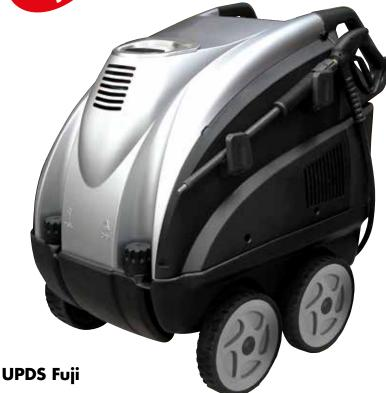
**Steam**: Vertical burner with high thermal efficiency steel coil. Auxiliary motor for burner. Discharge valve: allows a complete discharge of the boiler. Temperature regulator: the temperature is set up by an electronic regulator. Steam pressure gauge. Temperature regulator. Low fuel lamp. Double pipe gasoil pump. User friendly control panel. Unit can be continually refilled. Safety solenoid valve. Device for cleaning hot water mixed with steam.
