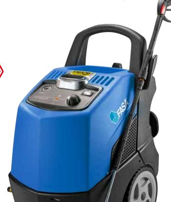
• 4 poles electrical motor (1450 RPM) with thermal protection and water cooling (three phase models). • Three ceramic coated pistons (1 ph), full ceramic pistons (3 ph), brass linear pump head with built-in by-pass valve.
