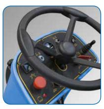
A 24 scrubbers are easy to use thanks to the simple and user friendly controls. From the control panel the operator can adjust the maximum forward speed and the quantity of cleaning solution outflow, selecting the options most suitable to the dirt type. Job is simplified and made faster by the automatic lifting of the squeegee and of the brush plate.
