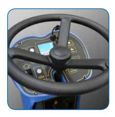
New control panel with digital controls and display. Digital display: with hour meter, battery charge level indicator, empty water tank level indicator and forward/reverse traction indicator. Speed control adjustment, horn, suction motor switch with delayed switch-off, brush plate lifting/lowering
